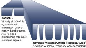
Inovonics Wireless 900Whiz Frequency Agile technology sends redundant information on a multitude of different channels across a 10MHz band to maximize range and readability.
